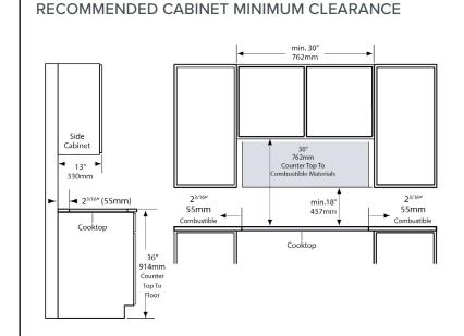
For optimal performance, the distance from the cooking surface to the bottom of the range hood should be between 24" and 30", unless otherwise noted. DO NOT install a range hood less than 24" above cooking surface.
