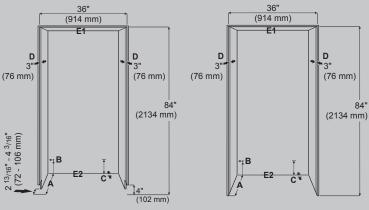
Cabinet depth frameless installation style = 25" (635 mm) Cabinet depth inset installation style = 25" (635 mm) + panel thickness
