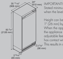
Stated minimum height dimensions include when the leveled feet are fully inserted.
